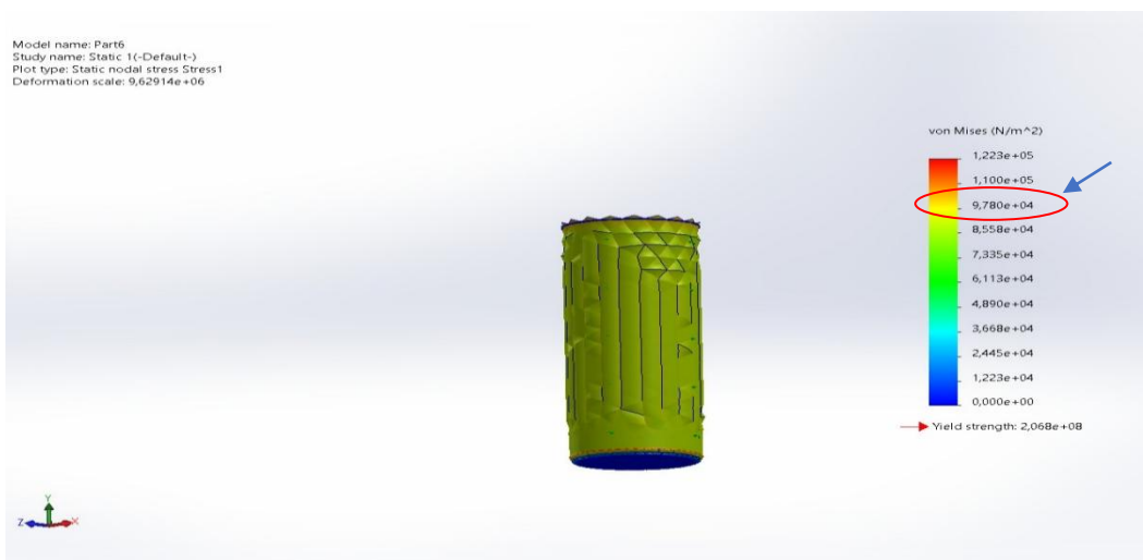
Figure 18 Simulation results of Von Misses stress for 3mm thick pressure cooker
