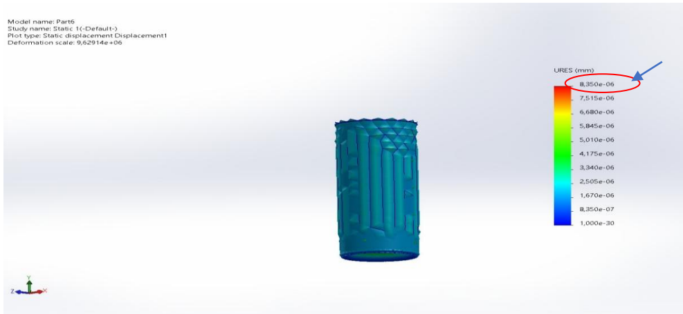
Figure 20 Displacement simulation results for 2 mm thick pressure cookers
