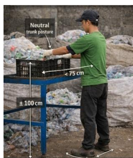
Figure 4. Ergonomically Designed Waste Sorting Workstation
