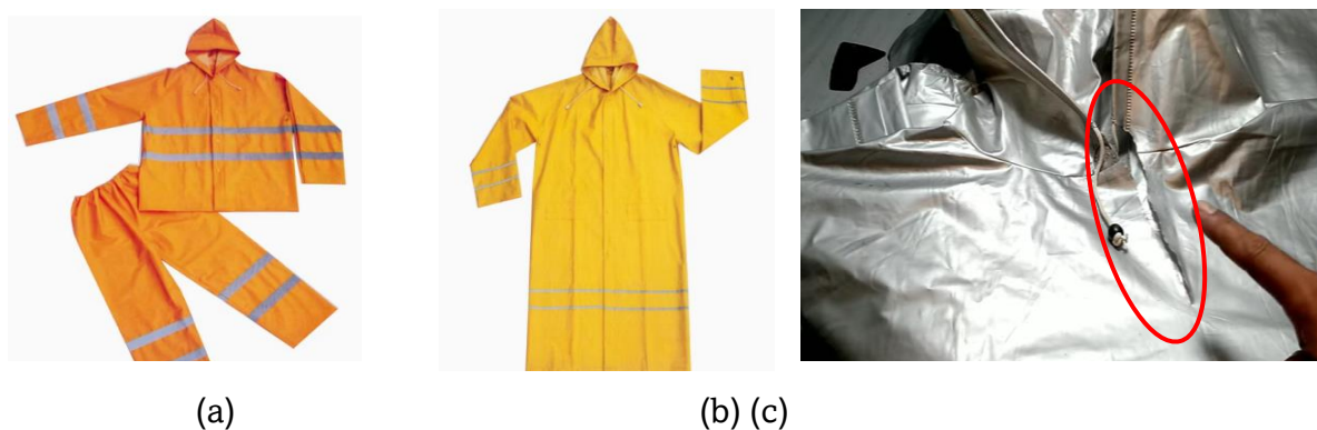
Figure 1.1 (a), (b) Raincoat made of polymer material (c) Torn raincoat (red circle)
