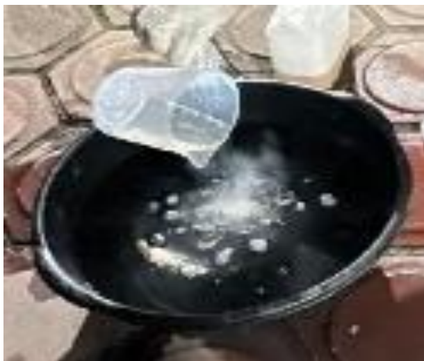
Figure 5. Aluminum slag mixing process with \text{H}_2\text{SO}_4 ) 10%
