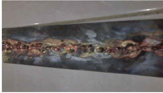
Figure 2. welding using copper welding wire filler on brass plates
