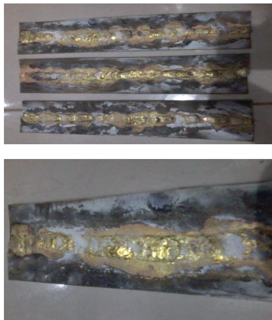
Figure 3. Welding using welding wire filler made from the brass mother itself
