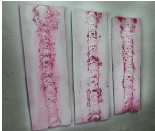
Figure 7. Penetrant Test Results on Welded Specimens
