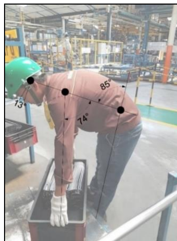
Figure 6. Angles of Worker A.'s Posture in Moving Activities at the Material Handling Station
