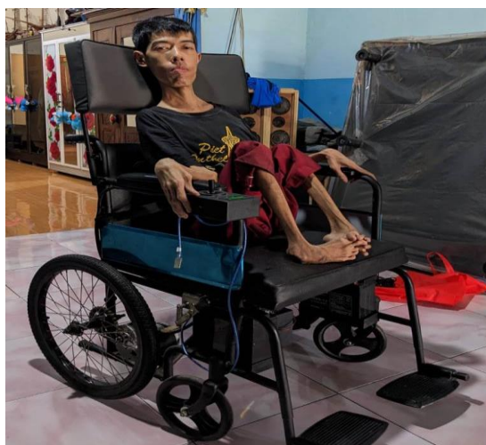
Figure 4 Electric wheelchair converted from Huda's manual wheelchair.
