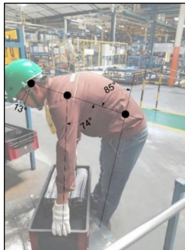
Figure 5. Angle of Worker A's Posture on Transferring Goods at the Material Handling Station
