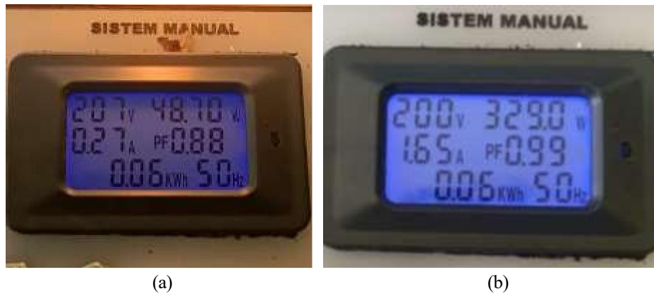
Figure 7 Measurement of Inductive and Resistive Loads on Manual Systems (a) Experiment 1; (b) Experiment 2
