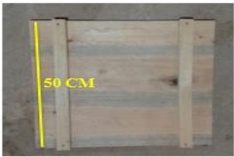
Figure 3. Design of the Square Core Section of the Round Tofu Press
